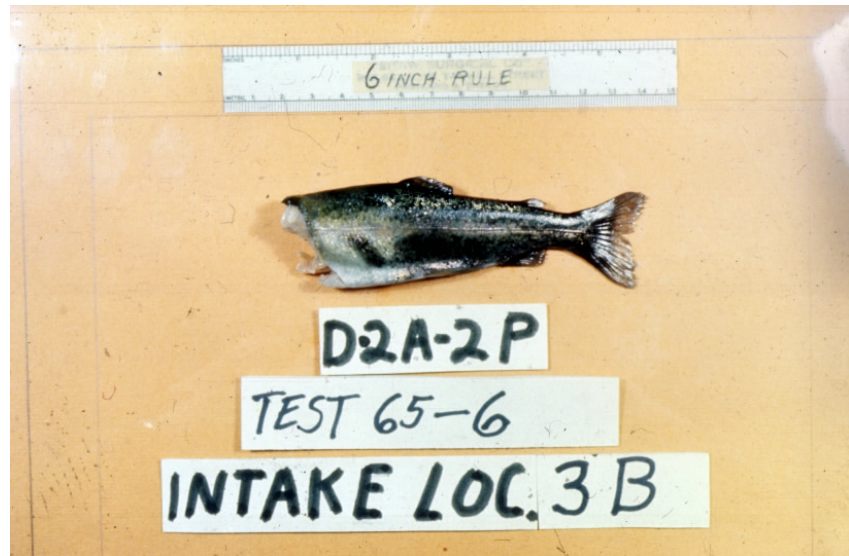
Figure 8: Juvenile Pacific salmon killed passing through a large diameter Kaplan turbine in a dam in the Columbia River, USA. In terms of damage to fish this site is equivalent to the likely equipment that would be deployed in the Severn Barrage.
