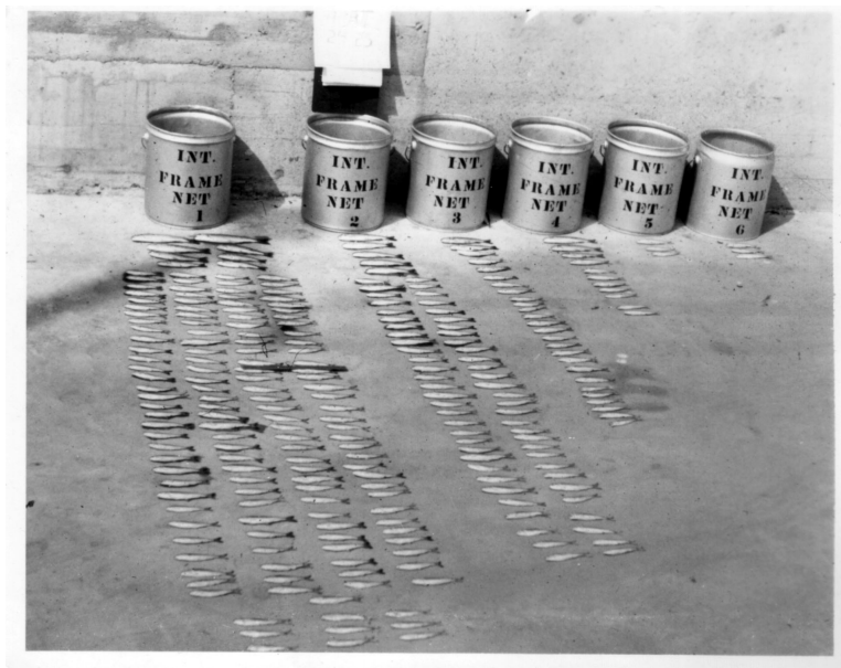
Figure 10: Catches of juvenile salmon from six nets positioned at different vertical positions in the intake of a dam on the Columbia river, net 1 being at the top and net 6 at the bottom, indicating the tendency for salmon smolts to be located in the upper layers of the flow.
