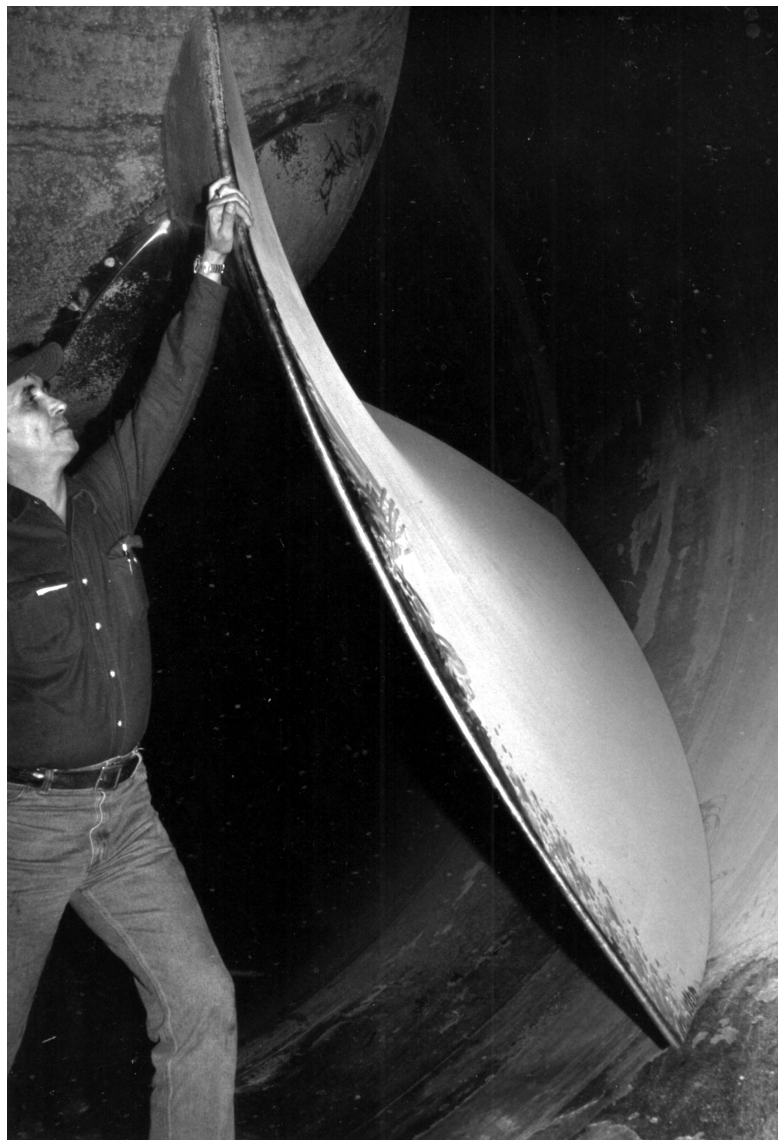
Figure 9: Leading edge of a runner blade of a 7.2 m diameter bulb turbine at Racine on the Ohio River, USA.
